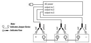
Three 12 VDC Batteries connected with a (2) series jumper for a 36 VDC Trolling Motor
